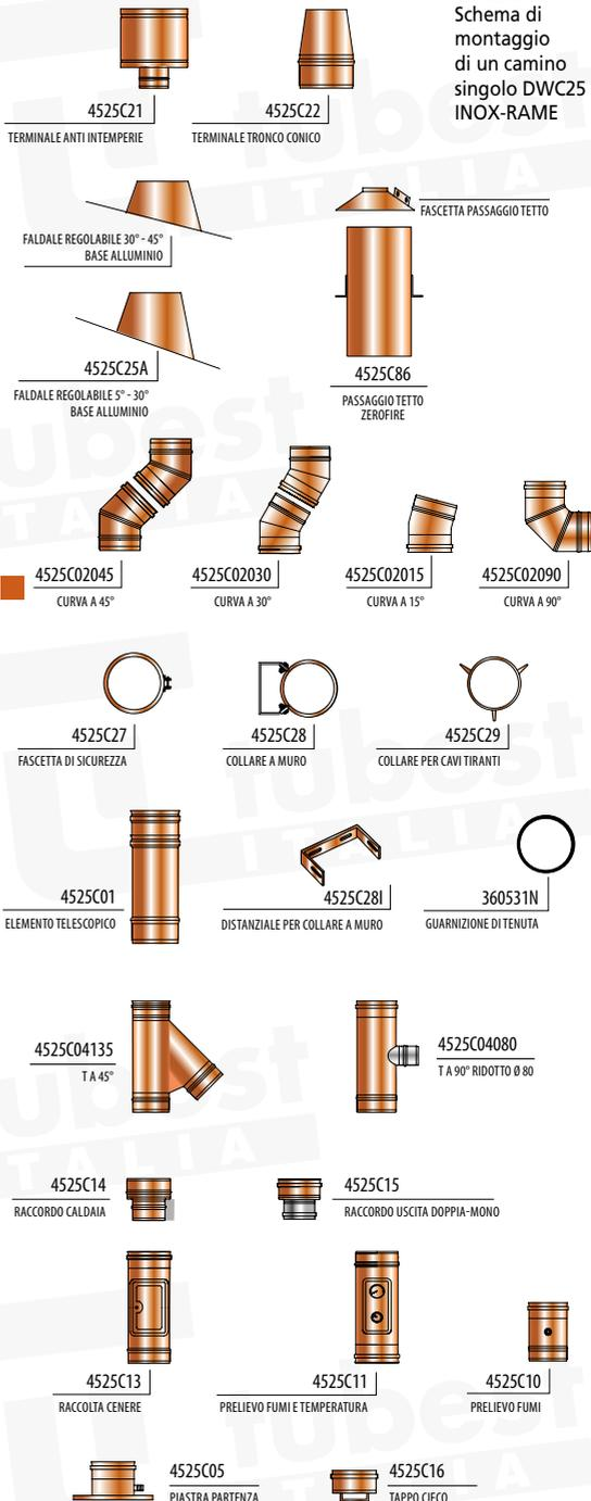
● MINIMO UN COLLARE A MURO OGNI 2 METRI
